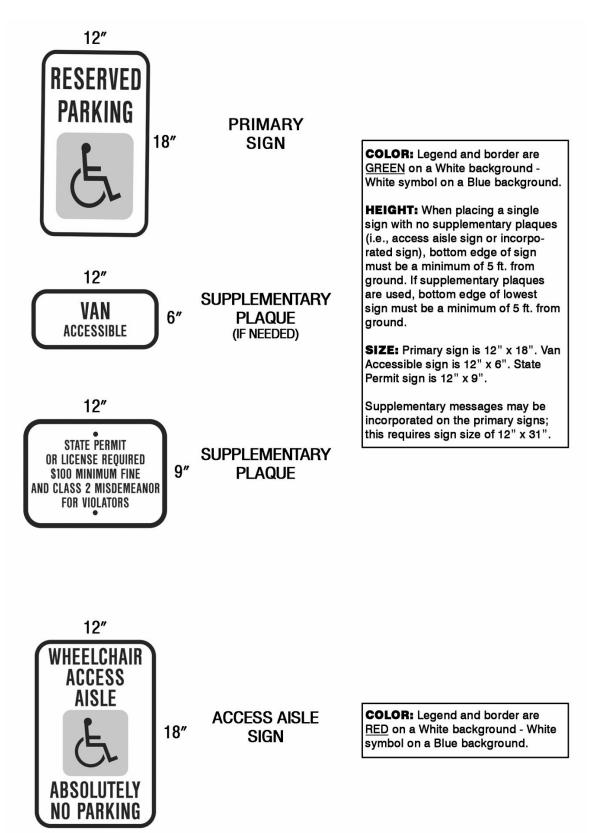
**1106.9** Access aisles and markings. Each access which is part of an accessible route shall extend the full length of the parking space it serves. The aisle must have diagonally striped markings spaced every 4 feet (1,219 mm). Boundaries of the access aisle must be marked. The end may be a squared or curved shape. Two parking spaces may share an access aisle.
